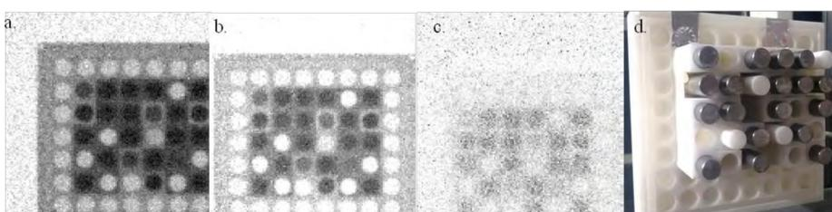
Radiographic images of a rectangular fuel assembly mockup, which is placed far (~45cm) from the detector using the ZnS converter (a), placed directly in front of the detector and using the ZnS screen (b), placed far (~45cm) from the detector using the BC400 converter (c) and a photo of it (d). 8x8 pixel binning have been applied.
