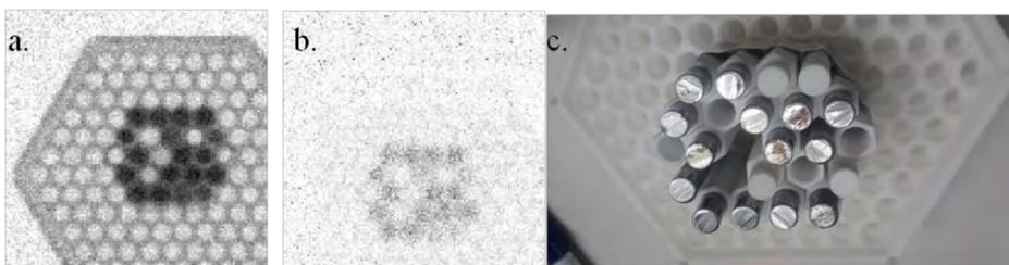
Radiographic image of a hexagonal fuel assembly mockup using the ZnS converter (a), the BC400 converter (b) and a photo of it (c). 8x8 pixel binning have been applied on the images
